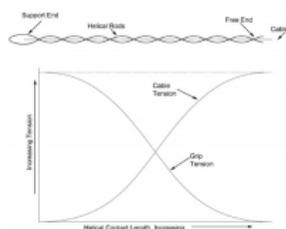
“Figure shows load transition from a cable to the helical grip”
