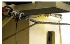
“PMI CABLE GRIP™ termination used to anchor a tow cable to the back deck of a vessel to perform load testing”
