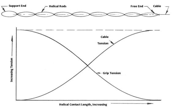
shown in the accompanying sketch. Radial compression increases while axial load in the cable decreases. This results is a combined effect that minimizes the chance of high stress concentration.
