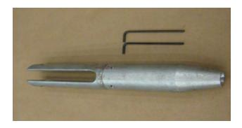
3. Insert the hex keys into the two holes in the base of the adaptor as shown until they bottom out.
