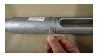
22. For attachment to equipment, use only the supplied PMI clevis pin. The termination assembly is now complete.
