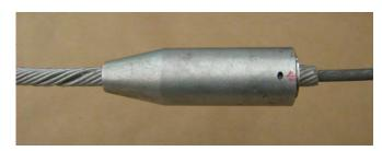
13. Clamp the housing in a vise and slide the adaptor over the cable toward the housing and the retainer, threaded end first. Place the hex keys in the adaptor holes as shown. Use the adaptor and hex keys as a spanner wrench to tighten the retainer firmly into the housing. The retainer is in correct position when it can no longer be screwed into the housing. When the retainer is properly in place there should be no looseness in the assembly.
