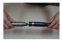
3. Screw BSR onto housing firmly by hand. Do not attempt to screw housing into BSR. Assembly is complete when BSR is threaded firmly on housing.
