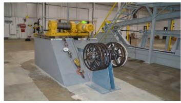
Long span tension setup
