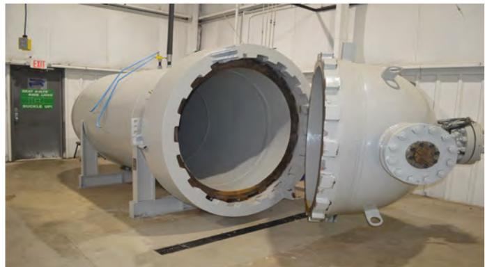
One of PMI's hydrostatic pressure chambers
