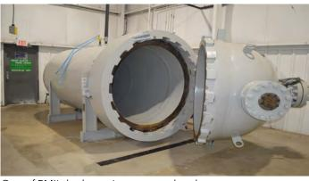
One of PMI's hydrostatic pressure chambers
