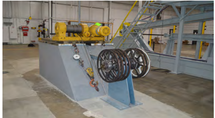
Long span tension setup
