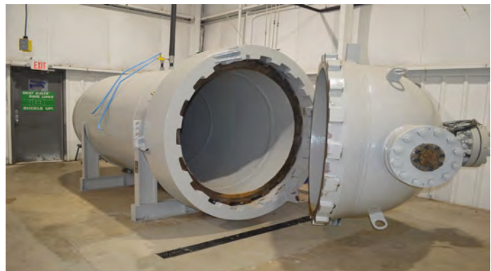
One of PMI's hydrostatic pressure chambers
