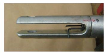
4. Clamp the housing in a vise. Unscrew the adaptor while keeping the hex keys pushed in until they engage the holes in the retainer. The retainer needs to be removed from the housing prior to any assembly. Note: There may be pre-applied antiseize compound on the threads of the adaptor, retainer and housing. Continue unscrewing the retainer until it is separated from the housing and set it aside.
